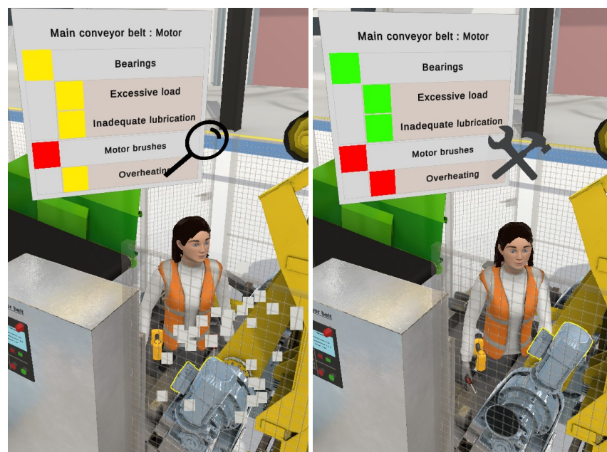
Fig. 5. The unloader failure has been triggered by an action in the scenario on an undisclosed component (the electric motor). The learner can visually and audibly notice the problem whereas the companion is alerted by the unloader smart object itself (left). Methodically checking the components enabled the problem to be isolated: a broken motor which was preventing the treadmill from operating (right).
